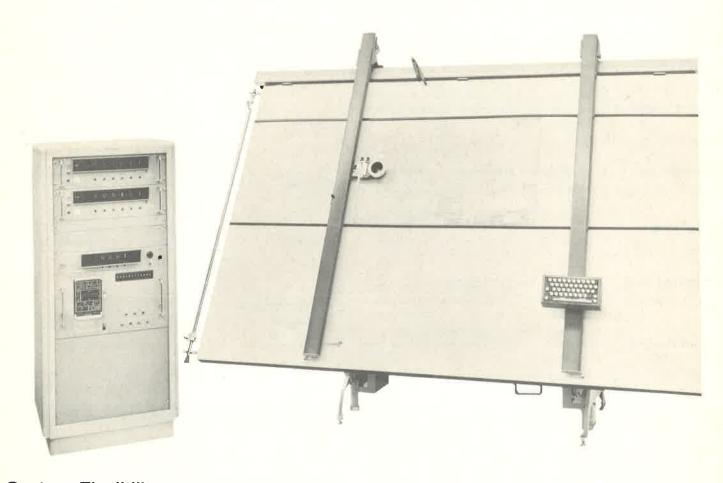
System Flexibility. The all new solid state LARR-V offers unequalled digitizing flexibility. Starting with the standard 48" x 60" usable digitizing area or with either of the optional  $(3' \times 3')$  or  $(4' \times 4')$ sizes the LARR-V can be customized to a particular application.
